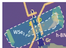
Fig. 1. Optical microscopy image of the fabricated WSe 2 /h-BN/Gr FGFET.
