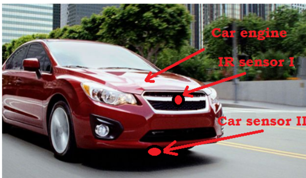
Fig. 1. Arrangement of thermal sensors (IR I and IR II) in the car
